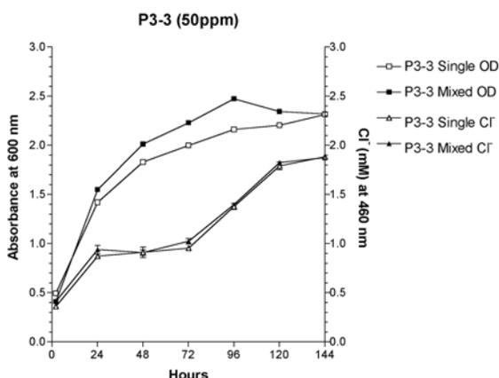
FIGURE 2 - Summary of chlorine release assays at 460 nm isolated from P<sub>3-3</sub> (50 ppm) plot as single vs. mixed indigenous culture with unknown microbes. The absorbance at 600 nm was to monitor culture growth.
