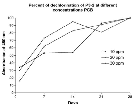
FIGURE 1- Summary of several tests (%) at different ppm levels (plot of P<sub>3-3</sub> soil sample). The chlorine release was expressed in percentages, 100% being complete dechlorination within 28 days. After 14 days the highest percentage of chlorine release was observed by microbes isolated from the 30 ppm-spiked soil sample.
