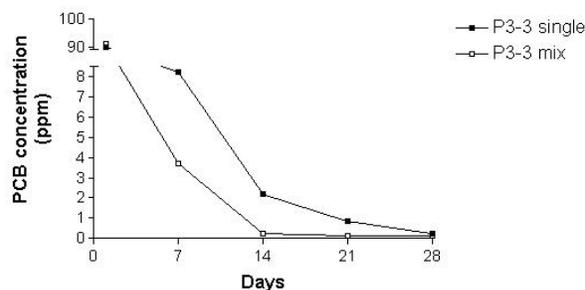
FIGURE 3 - Degradation of PCBs (Summary of several HPLC analyses; the mixed cultures degraded PCB within 14 days and single cultures within 28 days; mixed cultures were isolated from soil sample P<sub>3-3</sub> spiked with 100 ppm 2', 3, 4-PCB in the presence of alfalfa plants.
